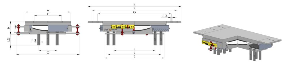
The above given sketch only for the illustration and the numbers of the screws and dowels / studs are to be read from the below given table. Please see I, J, F, G dimensions to consider the numbers of the screws. Example= J= 1x110 means 2 screws/dowels at this side with a distance of 110 mm. The above illustrated bearing, shows the bearing with elements, not included automatically in every offer. For scope of configuration offer description is relevant.
